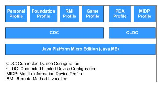
We describe the two configurations below. However, it is important to note that most developers will be working with interfaces provided at the profile level, and hence the configuration type does not necessarily play that important a role.
