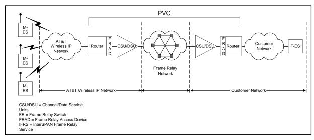
Figure 4: AT&T Wireless IP network connection to a frame relay network
