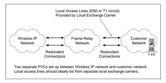
Keep in mind that for true redundancy, the two circuits that connect a customer's network to the frame relay carrier need to be independent, and should not pass through the same local carrier central office or traverse the same physical route. This can be accomplished by using separate local exchange carriers, if available.
