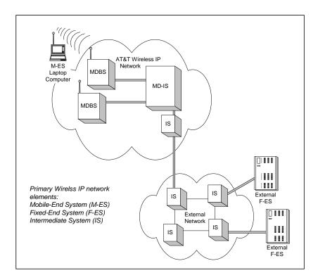
External F-ESs, which reside outside the AT&T Wireless IP network, are owned, operated, administered, and maintained by corporations or other entities outside the direct control of the AT&T Wireless IP network. In most cases, an F-ES is a traditional host system, server, or gateway that provides data or application services.
