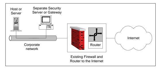
There are two fundamental types of wireless IP security solutions. One solution is packet filtering and port monitoring, which is implemented at the edge of the customer's network. The other is a virtual private network solution that involves implementing a secure "tunnel" across the Internet.
