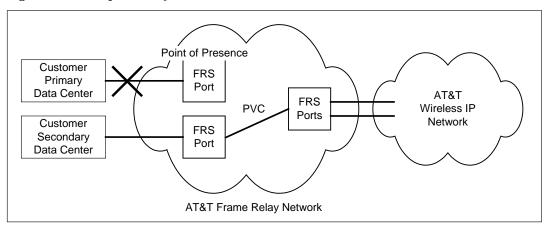
Figure 18: Backup PVC - After Site Failure
