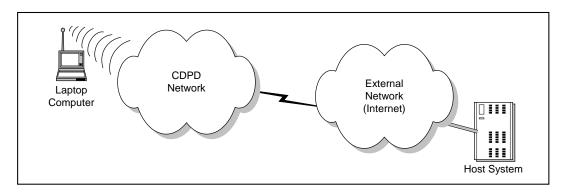
The options for connecting the AT&T Wireless IP network to a customer's internal data network includes using frame relay, the Internet, or leased-line connections. This paper describes the pros and cons of these options and presents important considerations regarding other pertinent topics, such as redundant connections, protocol considerations, number of mobile devices, message volumes, and router configuration.
