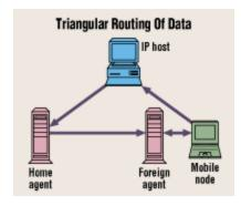
The home agent must know that the mobile node is legitimate, so security is an important issue with Mobile IP. Similarly, the mobile node must be able to trust the home agent. IPsec, a series of Internet security standards, can be used in conjunction with Mobile IP to provide authentication and encryption.
