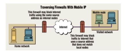
A similar problem can occur at the foreign network. Many firewalls are configured so that they will not pass datagrams from inside a network to the Internet if the source address differs from what is expected. The intent is to prevent the internal network from being a haven for malicious users spoofing source addresses and perpetrating mischief on the Internet. Unfortunately, the Mobile IP node's address does not belong on the internal network, so its transmissions may be blocked.
