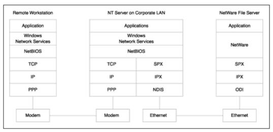
Figure 3: Accessing NetWare file server via intermediate server
