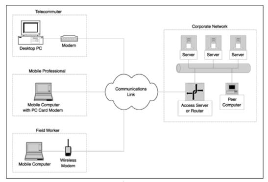
Figure 2: Elements of a remote computing solution
