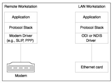
Figure 6: Comparison of remote node and LAN workstations
