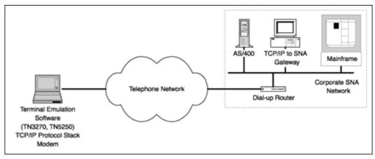
Figure 5: Accessing IBM hosts via a gateway.
